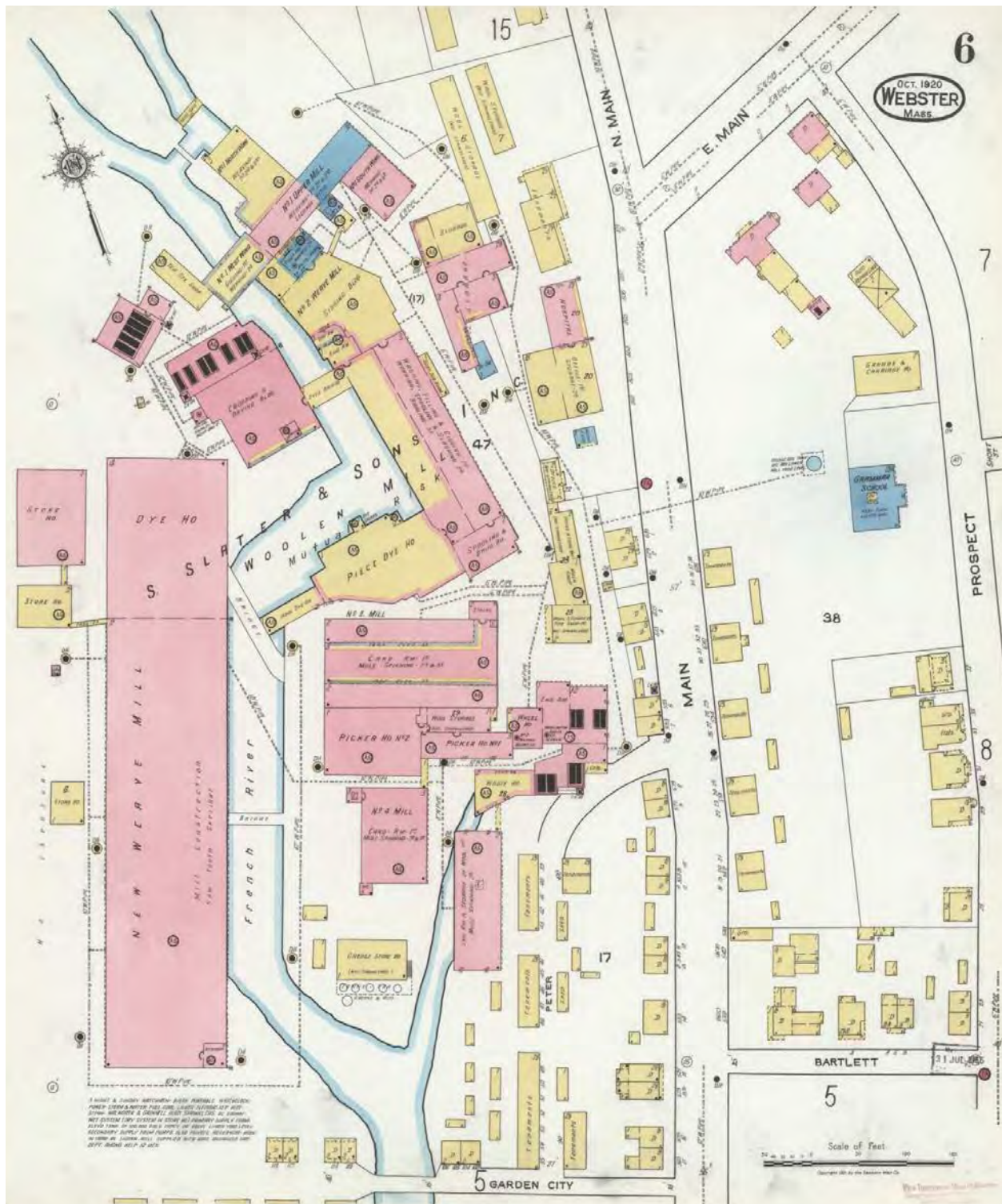
Sanborn map from 1920 showing the woolen mills in South Village. Brick buildings are shown in red, granite buildings are in blue, and wood buildings are in yellow. Sanborn maps from the 1920s and 1930s can be used to assess building and development through the end of the Slater mill period and the amount of building loss that the historic mill town has experienced since.
